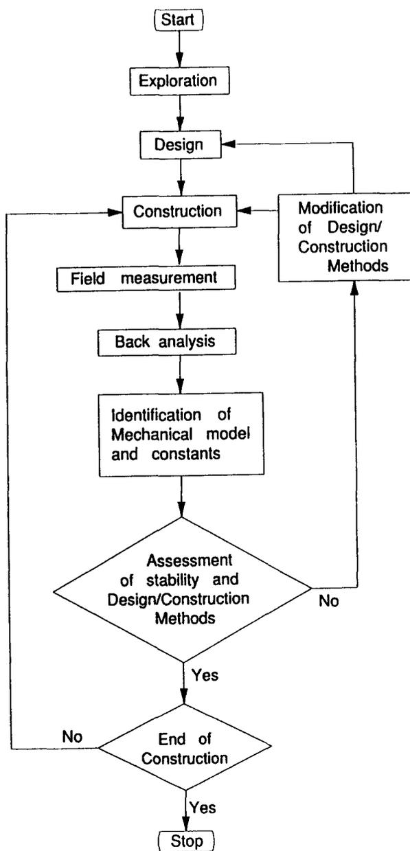
Figure 1. Procedure of assessing the design and construction methods.
