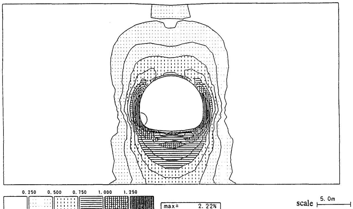
Figure 7. Maximum shear strain distribution (isotropic elastic model).
