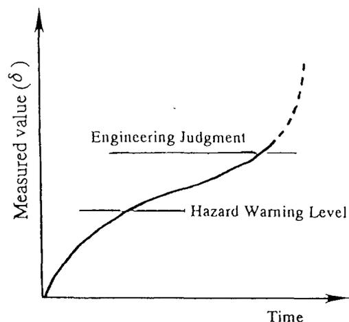
Figure 2. Schematic diagram for measured value in relation to hazard warning level.
