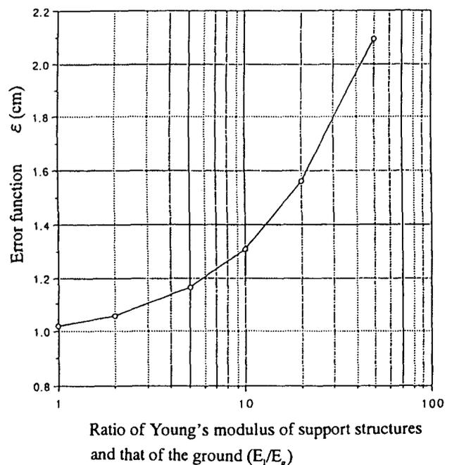
Figure 9. Error function plotted as a function of  $E_s/E_g$ .
