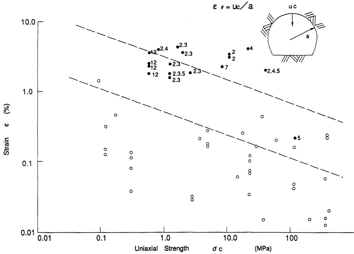
Figure 3. Relationship between the measured strain (obtained from crown settlement) and hazard warning levels.
