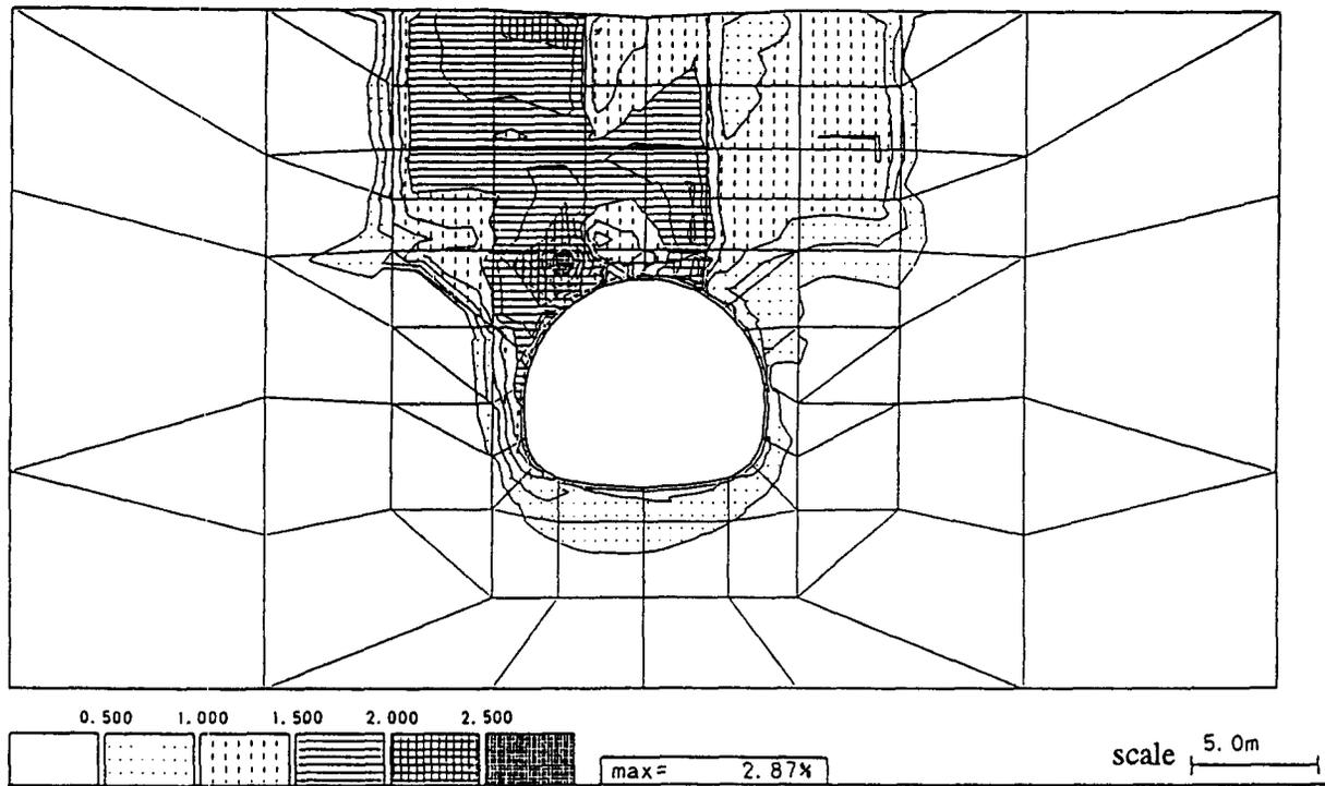
Figure 8. Maximum shear strain distribution (taking into account non-elastic strain).
