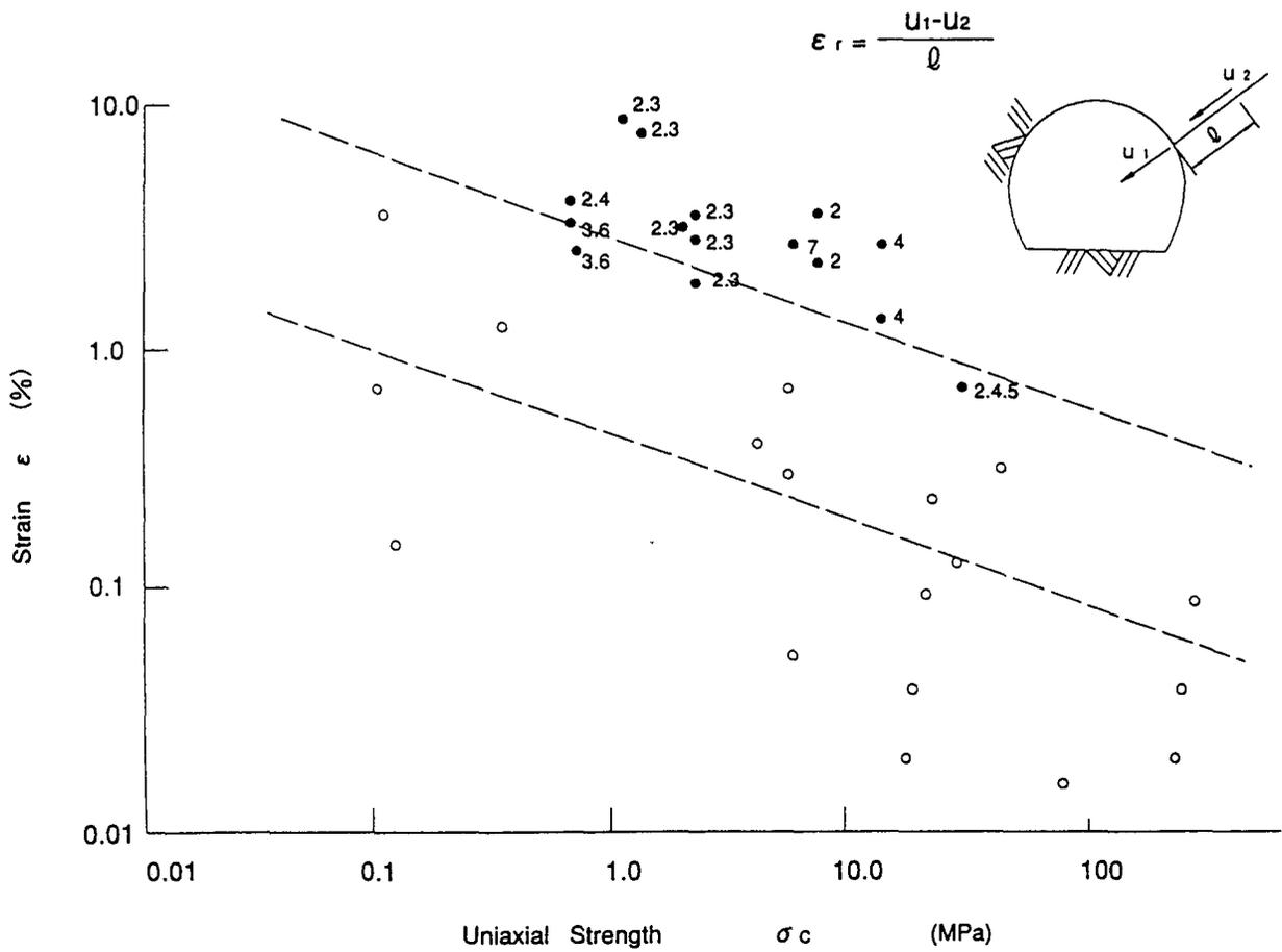
Figure 4. Relationship between the measured strain (obtained from extensometer measurement results) and hazard warning levels.
