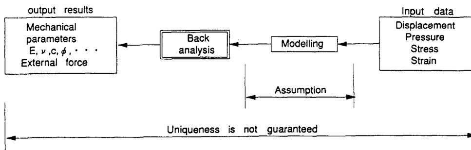
Figure 6. Comparison between the procedures of forward analysis and back analysis.
